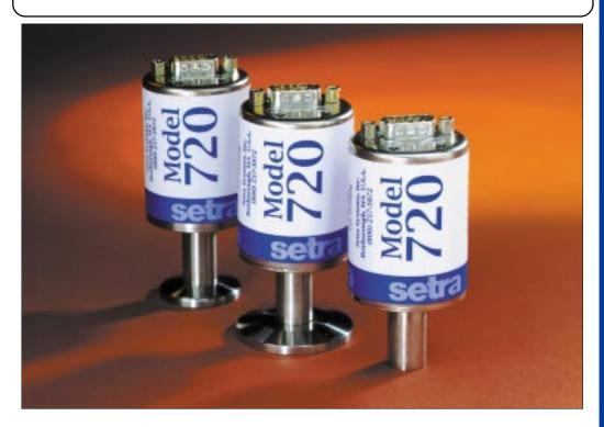
etra's Model 720 is an accurate, low cost pressure manometer for vacuum applications. The 720 is designed to be used with pressure media compatible with Inconel®. The all-welded construction eliminates stability issues inherent in other designs due to frictional contact between dissimilar metals.
