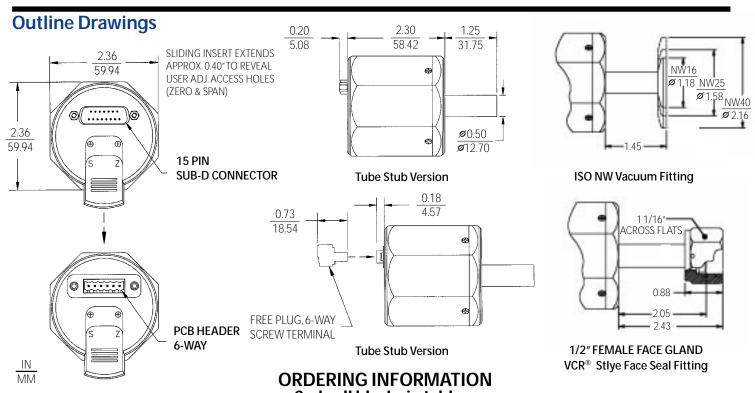
**Code all blocks in table. Example**: Part No. 7601010TAN17CD2A for a 760 Transducer, 10 Torr Range, ISO NW16 Fitting,
