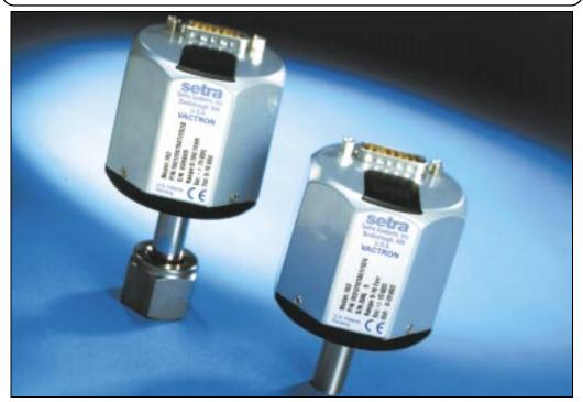
etra's Vactron Model 760 capacitance manometer is an absolute pressure transducer designed for accurate and repeatable vacuum measurements. Various full scale ranges are available from 10 Torr up to 1000 Torr. The units of measurement may be specified in Torr, mBar/hPa, kPa or psia.
